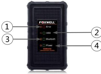
Figure 2-5 Front View of VCI dongle
